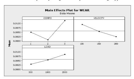
Figure 4. Effect of control factors on wear rate
