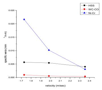
Figure 5. Effect of speed on specific wear rate for various compositions
