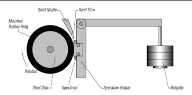
Figure 3. Dry Sand Rubber/Wheel Abrasion Test
