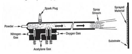
Figure 1. Schematic of Detonation Gun Process
