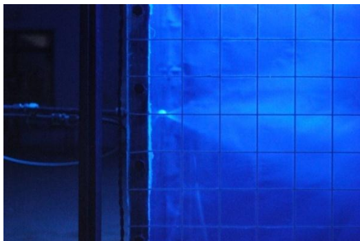
Figure 9. Spray for \alpha = 60^\circ and \Delta P = 12 bar
