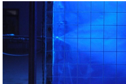
Figure 8. Spray for \alpha = 60^\circ and \Delta P = 15 bar
