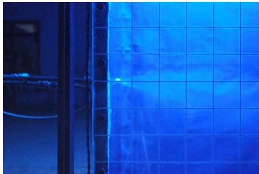
Figure 11. Spray for \alpha = 60^\circ and \Delta P = 6 bar
