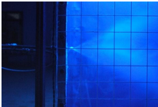
Figure 7. Spray for \alpha = 60^\circ and \Delta P = 18 bar
