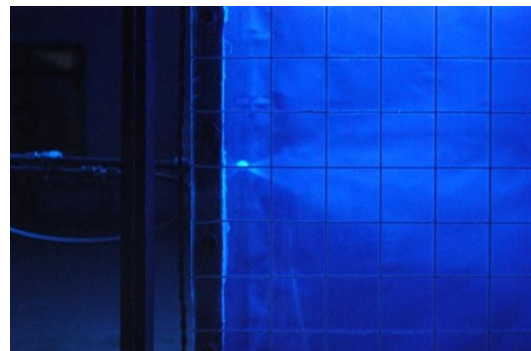
Figure 10. Spray for \alpha = 60^\circ and \Delta P = 9 bar
