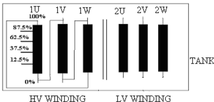
Figure 3 Diagrammatic representation of three-phase Transformer Winding.
