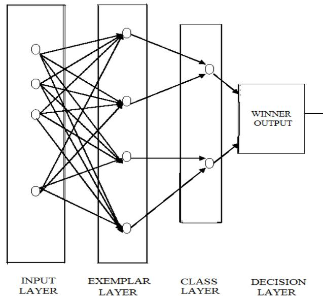
Figure 1 Architecture of Probabilistic Neural Network
