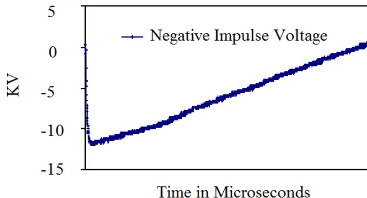
Figure 5 Lightning Impulse Voltage Waveform
