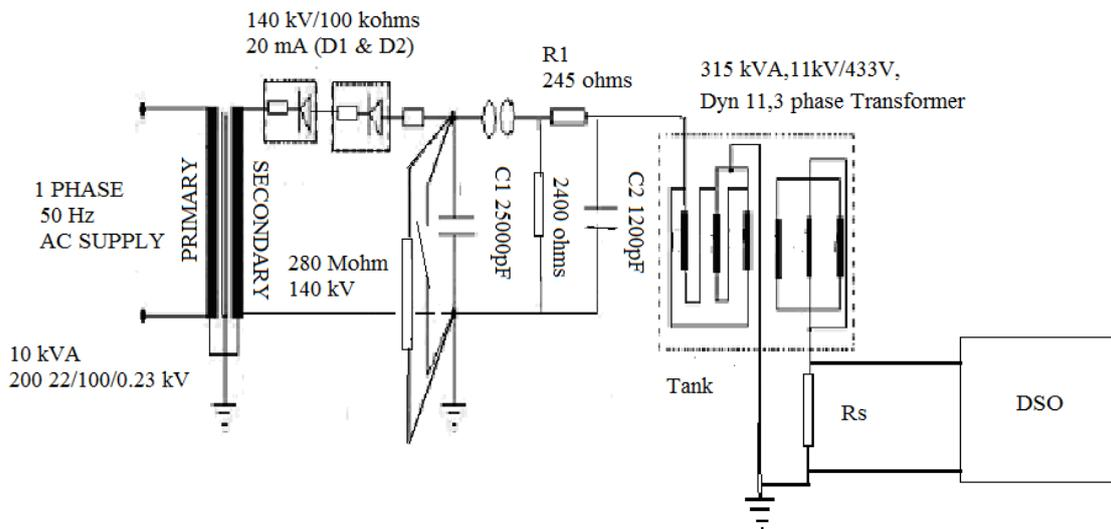
Figure 4 Electrical test set-up
