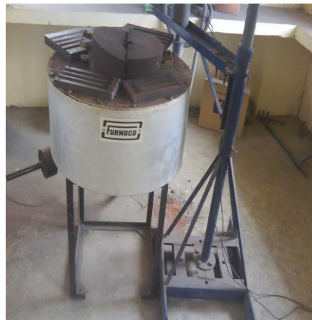
Fig.1: External View of Electrical Resistance Furnace
