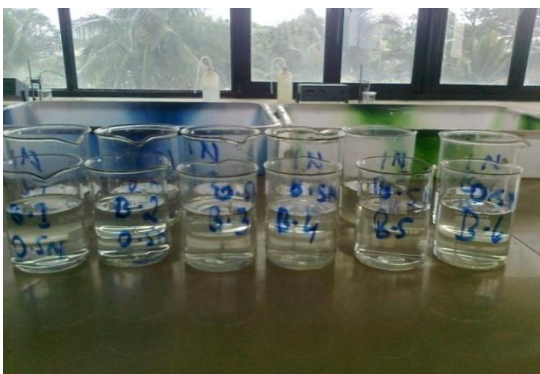
Fig 2: Test Specimens in Hcl solution
