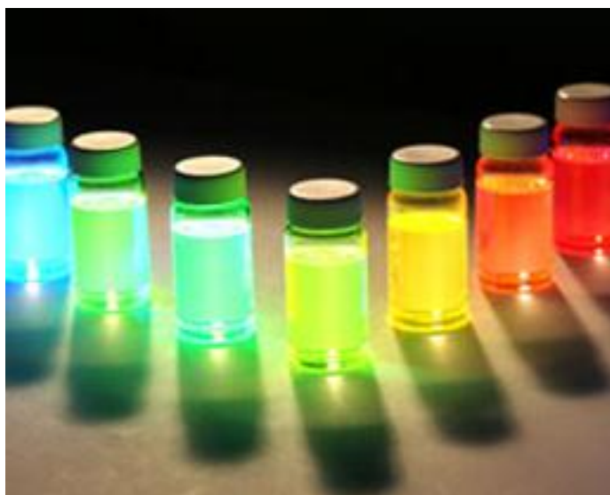
Fig.1 Quantum dots arranged by size, emitting light of different colours
