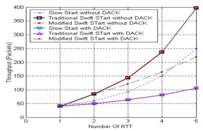
Figure 11 Throughput versus Number of RTT for (RTT=0.1 Sec, C=1544000 Bps)
