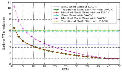
Figure 12 Number of RTTs which is needed to reach ssthresh Versus RTT/τ.
