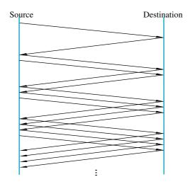
Figure 1 Packets in Transit during Additive Increase: Add one Packet each RTT.
