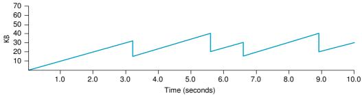
Figure 2 Typical TCP sawtooth pattern.
