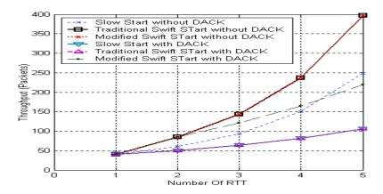
Figure 10 Throughput versus Number of RTT for (RTT=0.1 Sec, C=1544000 Bps)
