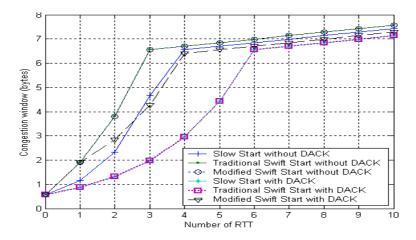
Figure 9 Congestion Window versus Number of Roundtrip Times for (RTT=0.1 Sec, C=1544000 Bps).
