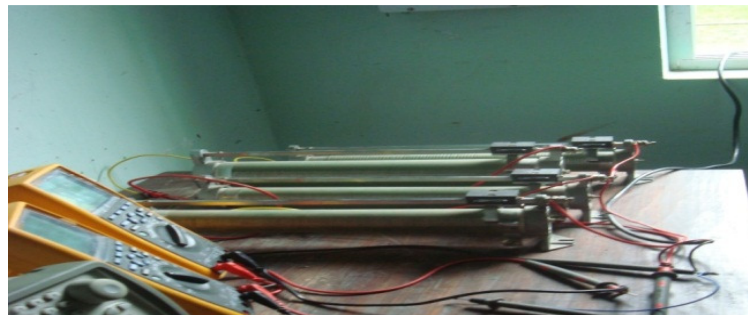
Figure 2. Arrangement for collecting data from the PV module
