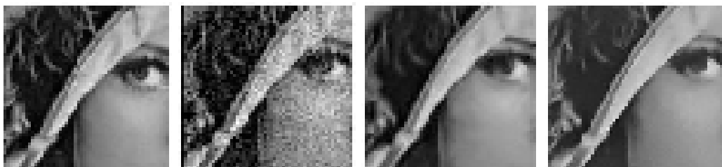
Figure 4. Comparison between non-local method and fast non-local denoising method result. From left to right, original image, noised image, result of non-local (MSE 60) and result of fast non-local (MSE 72)
