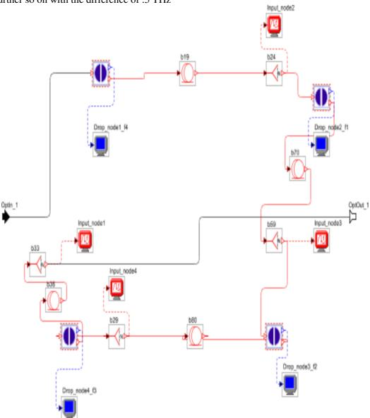
**Figure 1.2:** Set up for ring optical network
