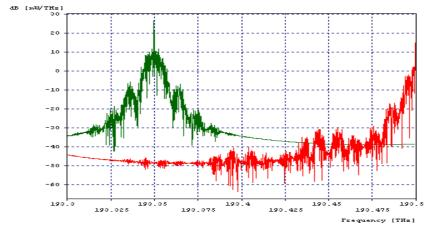
Figure 1.10: Optical Spectrum at node 2 before and after transmission
