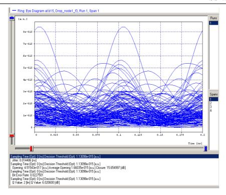
Figure 1.3: Eye diagram for Node 1
