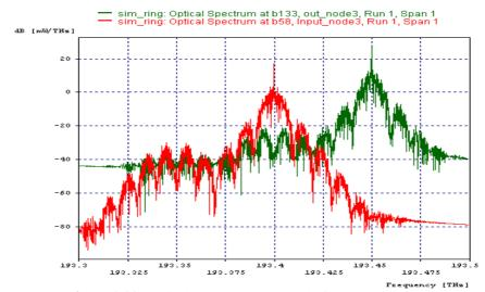
Figure 1.11: Optical Spectrum at node 3 before and after transmission
