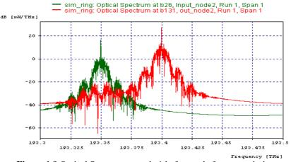
Figure 1.9 Optical Spectrum at node 1 before and after transmission
