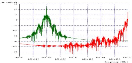
Figure 1.12: optical spectrum at node 4 before and after transmission
