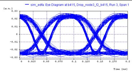
**Figure 1.5** Eye diagram for Node 3
