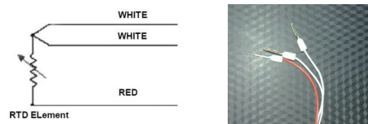
Figure 3. RTD sensors with line diagram
