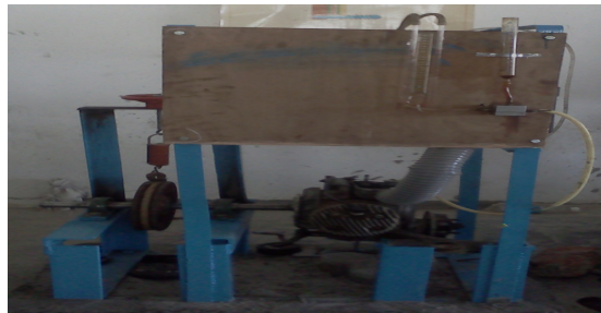
Figure 1 Experimental setup for the effect of methanol -gasoline, ethanol-gasoline and n-butanol-gasoline blends
