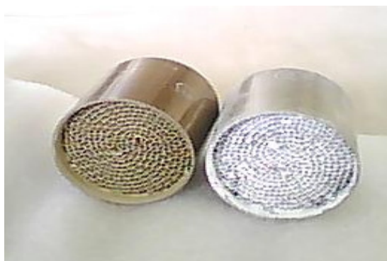
Fig 2.0 Pt-Rh catalytic converter (Left), ZrO_2 catalytic converter (Right)
