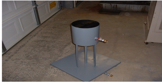
Figure 2 - Jominy End Quench Test apparatus
