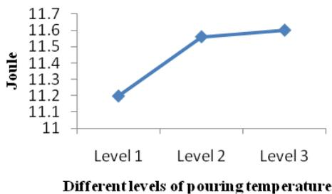
**Fig. 9** Variation of impact strength with the levels of process parameter ‘C’
