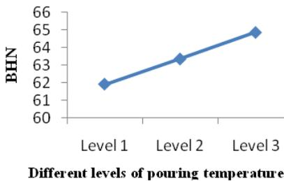
**Fig. 5** Variation of hardness with the levels of process parameter ‘C’
