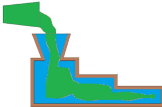
**Fig. 1** Acetone dropped over the pattern coated with Plaster of Paris
