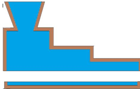
**Fig. 2** Two parts of pattern with coating
