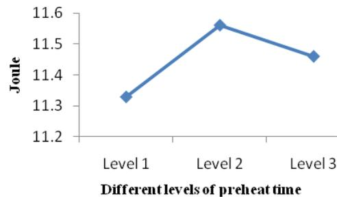
**Fig. 10** Variation of impact strength with the levels of process parameter ‘D’
