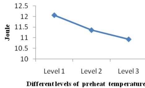
**Fig. 8** Variation of impact strength with the levels of process parameter ‘B’
