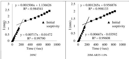
Figure 5 Water absorption in mm versus square root time
