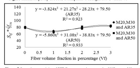
Figure 7 Secondary sorptivity of PFRC x compressive strength of NC versus Vf
