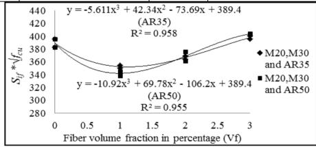
Figure 6Initial sorptivity of PFRC x compressive strength of NC versus Vf
