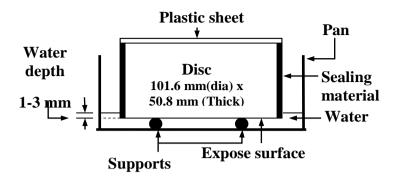
Figure 1Schematic sorptivity test set-up
