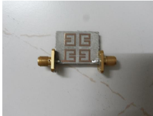
Fig.7. A fourth-order double-fold hairpin line microstrip bandpass filter of dimensions of 144 mm 2
