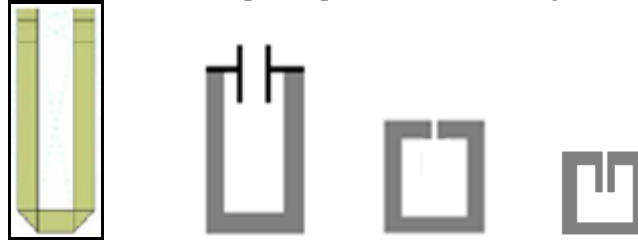
Fig 1. Actual, capacitor loaded, single-fold and doublefold hairpin line microstrip resonators
