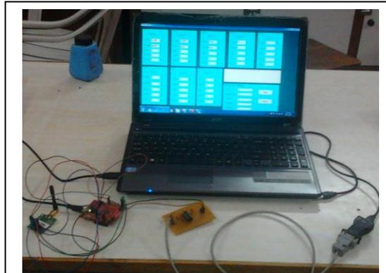
**Figure.13** The Base Station continuously presenting the values of humidity and temperature of the polyhouse Environment.
