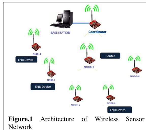
**Figure.1** Architecture of Wireless Sensor Network
