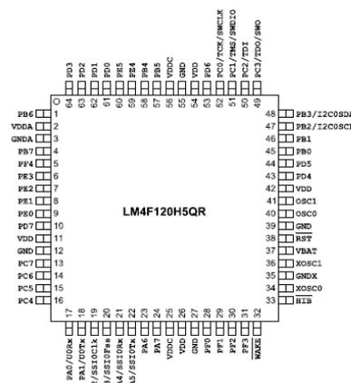
Figure.5 Pin Diagram of LM4F120H5QR
