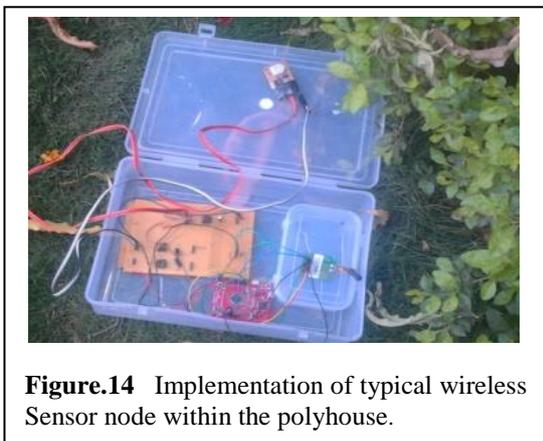
**Figure.14** Implementation of typical wireless Sensor node within the polyhouse.
