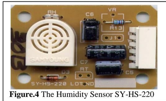
Figure.4 The Humidity Sensor SY-HS-220
