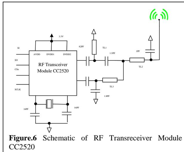
IEEE 802.15.4 standards [26] within the 2.4 GHz unlicensed ISM band. The figure 6 depicts schematic of the RF module CC2520. This chip enables industrial grade applications by offering up to 125°C and low voltage operation. In addition, CC2520 provides extensive hardware support for frame handling, data buffering, burst transmission, data encryption, data authentication, clear channel assessment etc. The RF module CC2520 transceiver has following features:
