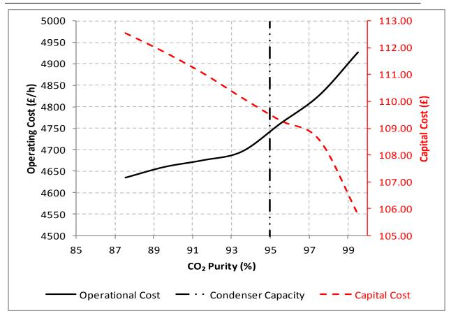
Figure 1: Capital and Operating cost variation during CO2 Purity in stripper top optimisation
