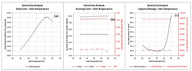
Figure 7: Sensitivity analysis of the CCS plant with respect to the flue gas inlet temperature
