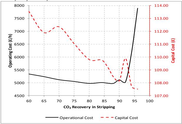
Figure 2: Capital and Operating cost variation during CO2 recovery in stripping optimisation
