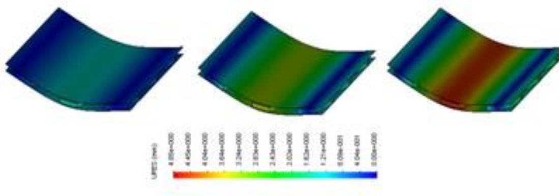
**Figure 7.** Deflection plots for various loads with core height of 5mm
