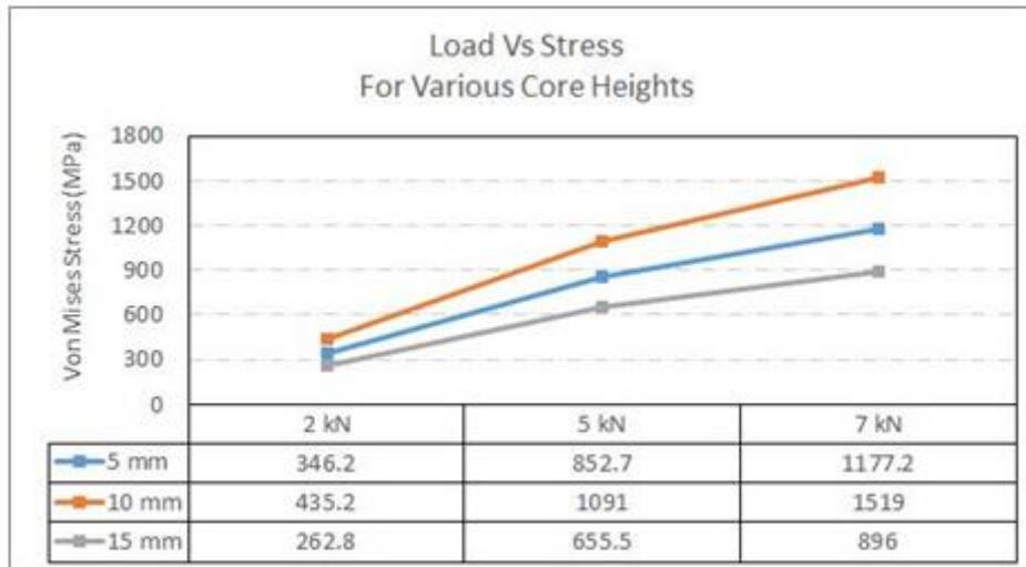
Figure 9. Variation of Von Mises Stress with core height.
