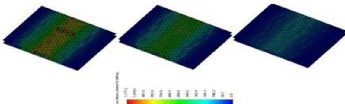
**Figure 8.** Stress distribution for various loads with core height of 5mm
