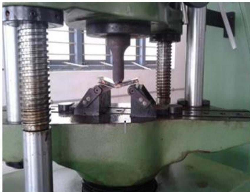
Figure 5. Specimen Loaded and Tested using UTM
