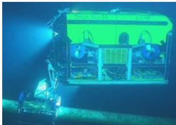
Figure 4: ROV measuring the thickness of a duct using ART. Adapted from [6].
