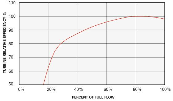
Fig. 5 Turbine Efficiency with full flow
