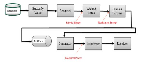
Fig 2. Schematic View of a Hydro Power Plant.
