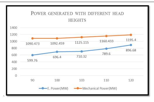
Fig 4: Power generated with different head height
