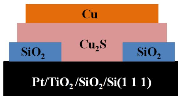
Fig. 1. A typical structure of memory device cell
