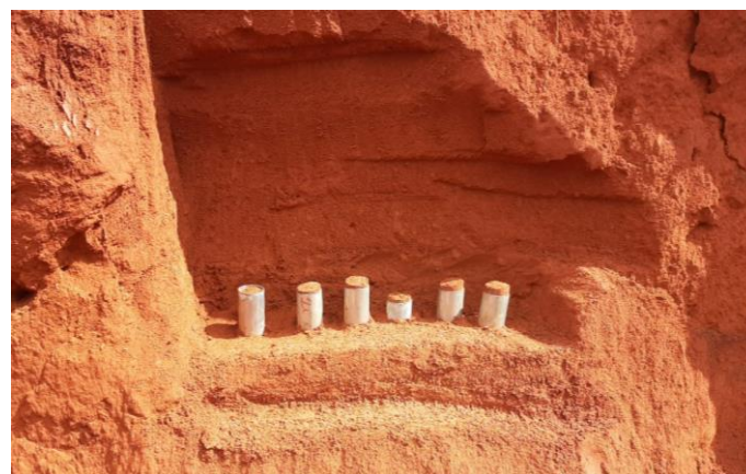
Figure 12. Sandy clay layer present at the investigation site (collapsible soil). The cylinders in the center of the image are the molds used to collect the material.
