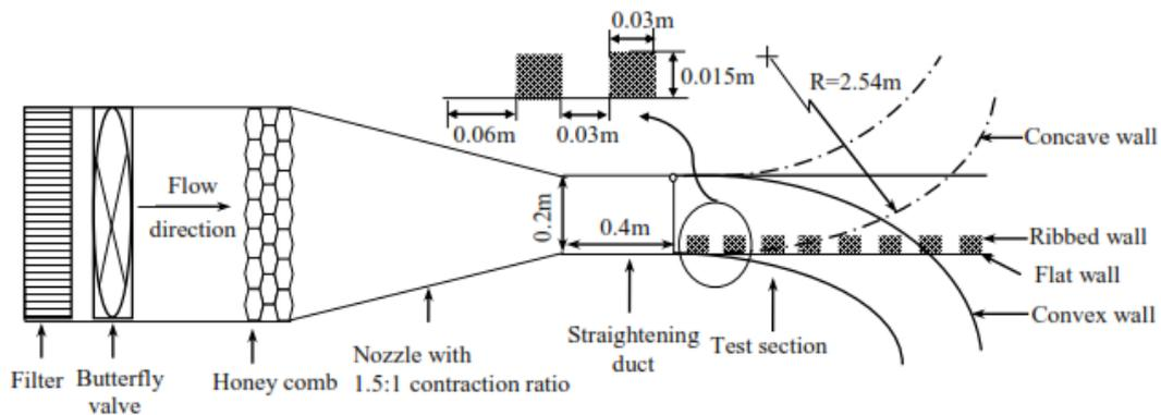
Figure 1. Wind tunnel and test section
