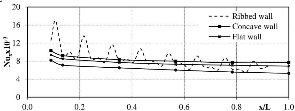
Figure 5. Local Nusselt numbers over the flat, concave, convex and ribbed walls at  $Re_x=4.5 \times 10^6$
