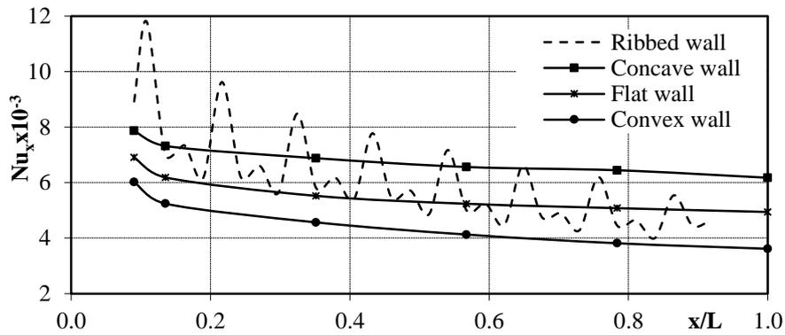
Figure 4. Local Nusselt numbers over the flat, concave, convex and ribbed walls at  $Re_x=3.1 \times 10^6$ .
