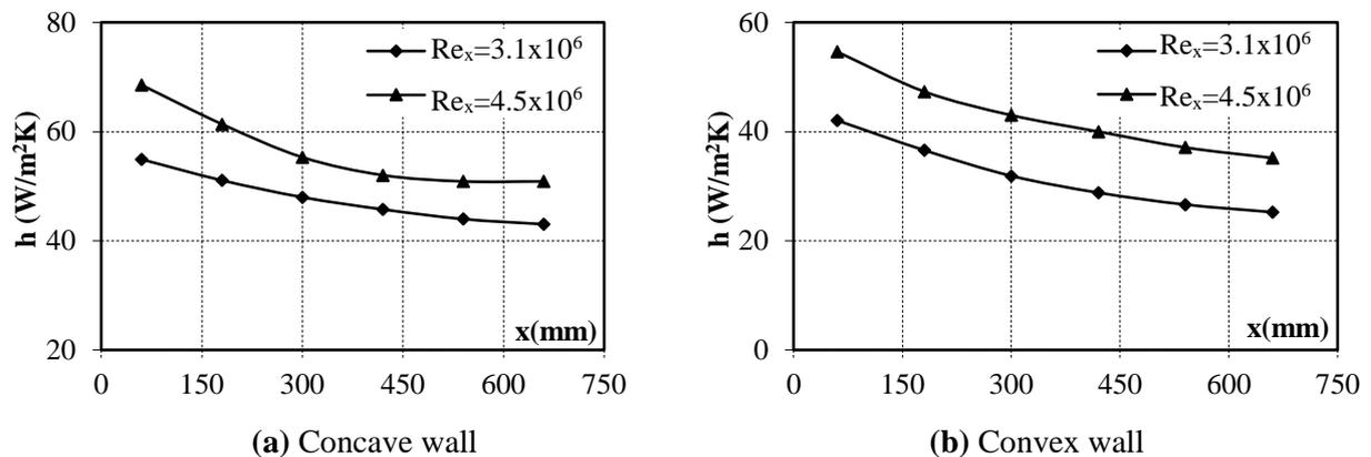
**Figure 2.** Streamwise variation of the heat transfer coefficient over the concave and convex wall
