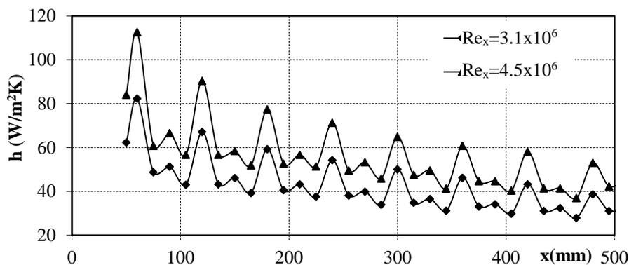
**Figure 3.** Streamwise variation of the heat transfer coefficient over the ribbed wall
