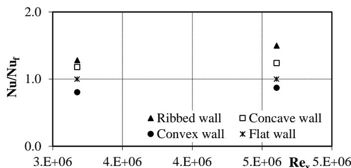
Figure 6. Variations of  $Nu/Nu_f$  with  $Re_x$  over the flat, concave, convex and ribbed walls.
