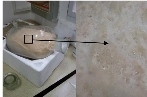
Fig.2 The reaction between egg shells and HCl acid
