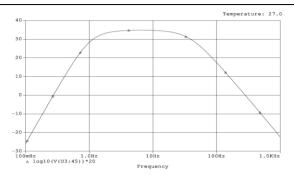
Figure 4. Frequency response of the active filter.
