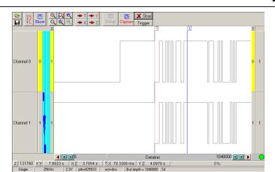
**Figure 6.** Testing stage by using a Lu-La Logic Analyzer. Channel 0 and 1 show the receiver output and transmitter input, respectively.
