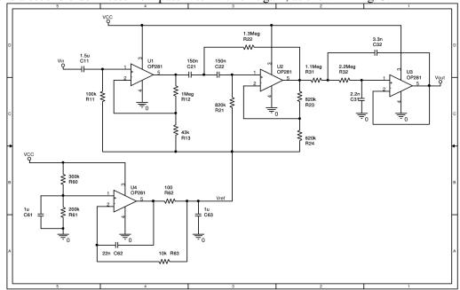
Figure 3. Band-pass active filter.
