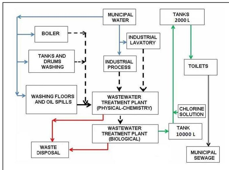
Figure 6 - System modification with reuse of wastewater for toilet
