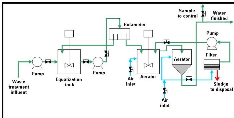
Figure 2 - Effluent treatment plants (biological treatment).
