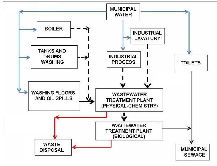
Figure 5 - Flowchart of the treatment and disposal of wastewater
