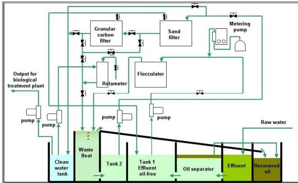
Figure 1 - Effluent treatment plants (physical-chemical).
