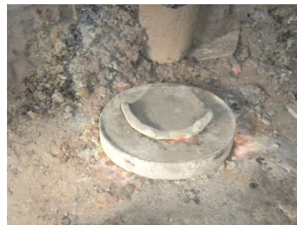
Figure 3: A pit furnace melts the A713 Aluminium alloy
