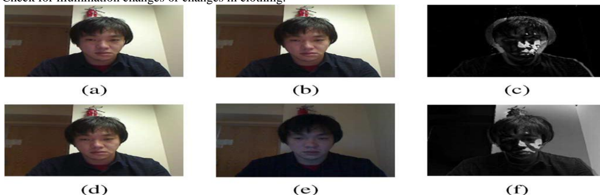
Figure 3. Example of image subtraction for illumination change detection. The difference image in (f) shows an illumination change between (d) and (e), but the difference image in (c) does not show change in illumination between (a) and (b).
