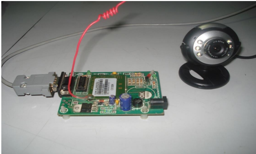
Fig 3.18: Device using for motion detection and alerting
