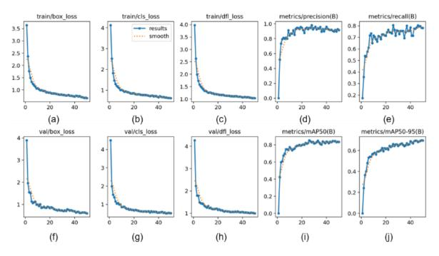
Figure 7 – Results comparing the performance metrics of precision, recall, mAP 50% and mAP 50-95% for the YOLOv8 small algorithm.
