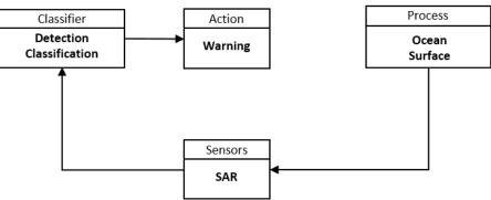
Figure 1 - Schematic of the proposed system for detecting oil slicks on the ocean surface.
