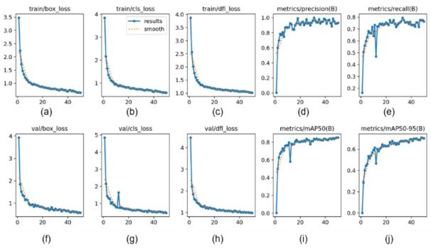
Figure 6 – Results comparing the performance metrics of precision, recall, mAP 50% and mAP 50-95% for the YOLOv8 nano algorithm.
