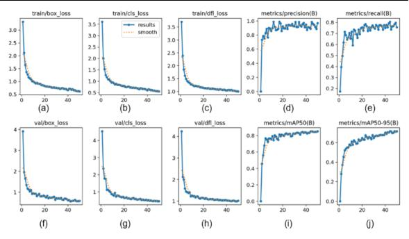
Figure 8 – Results comparing the performance metrics of precision, recall, mAP 50% and mAP 50-95% for the YOLOv8 medium algorithm.
