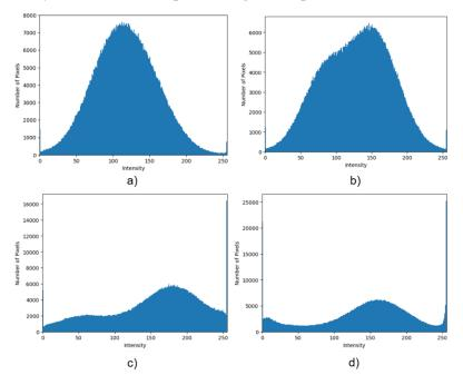
Figure 6 – Histogram of pixels in relation to image classes: (a) and (b) represent the class with oil stains; (c) and (d) represent the class without oil stains.
