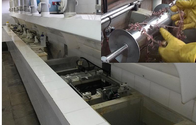
Figure 6: Recipients used in the electroplating process; detail of the parts manually handled in a rotary reel.
