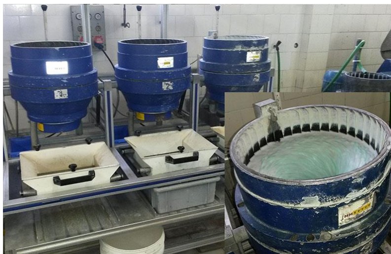
Figure 4: Second stage of finishing with plastic abrasives based on oxide, silicate and carbonate in rotary tumblers.
