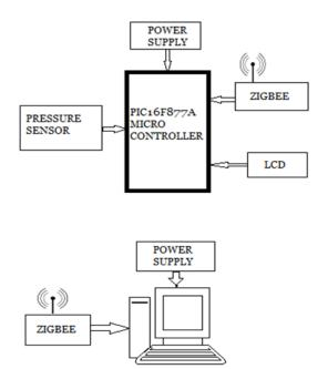
Figure 1: Functional Block of the System
