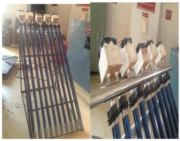
Figure 2: arrangement of solar tubes for hot air
