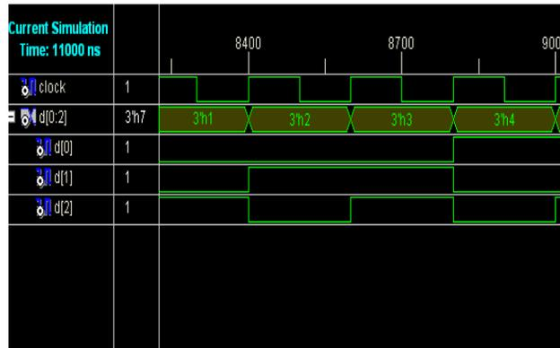
Fig. 2 Simulation of an UP counter
