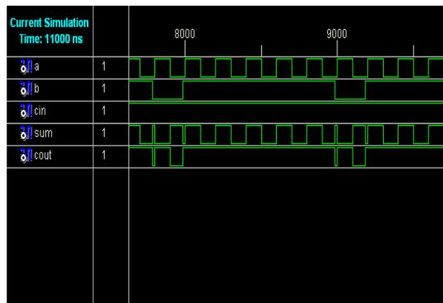
Fig. 1 Simulation of an Adder circuit
