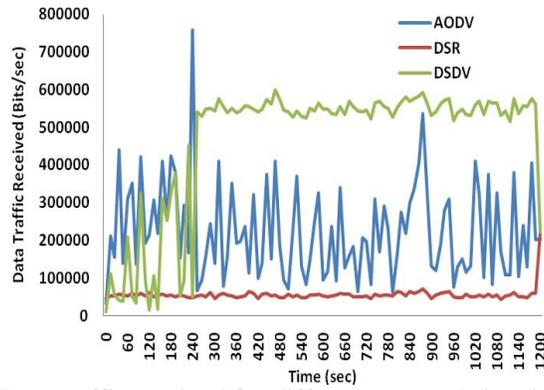
Figure 5: Data traffic received for different protocols in wireless LAN
