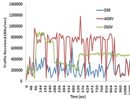
Figure 3: Control traffic received for different protocols in wireless LAN
