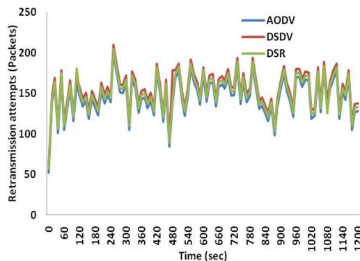
Figure 8: Retransmission attempts for different protocols in wireless LAN
