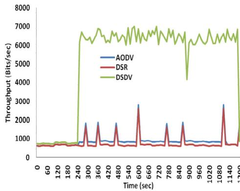
Figure 7: Throughput of different protocols in wireless LAN
