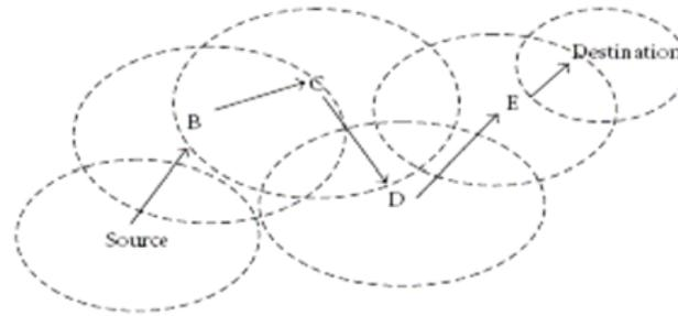
Figure 1: Ad-hoc networking model
