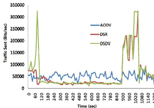
Figure 4: Control traffic sent for different protocols in wireless LAN
