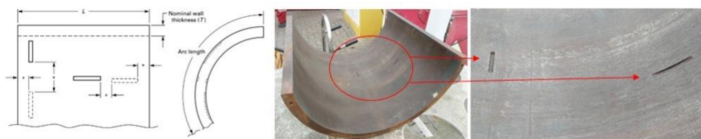
Figure 2. Girth weld calibration block
