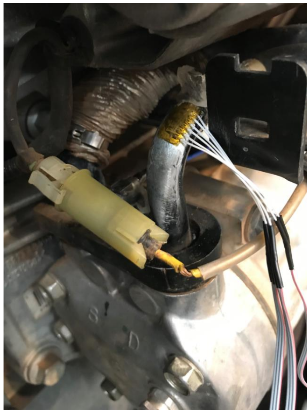
Figure 3. Rosette strain gauge attached to the interested region
