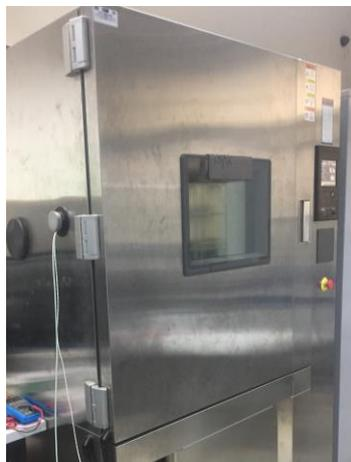
Figure 3 - Platinous EPL-4H series climatized chamber.
