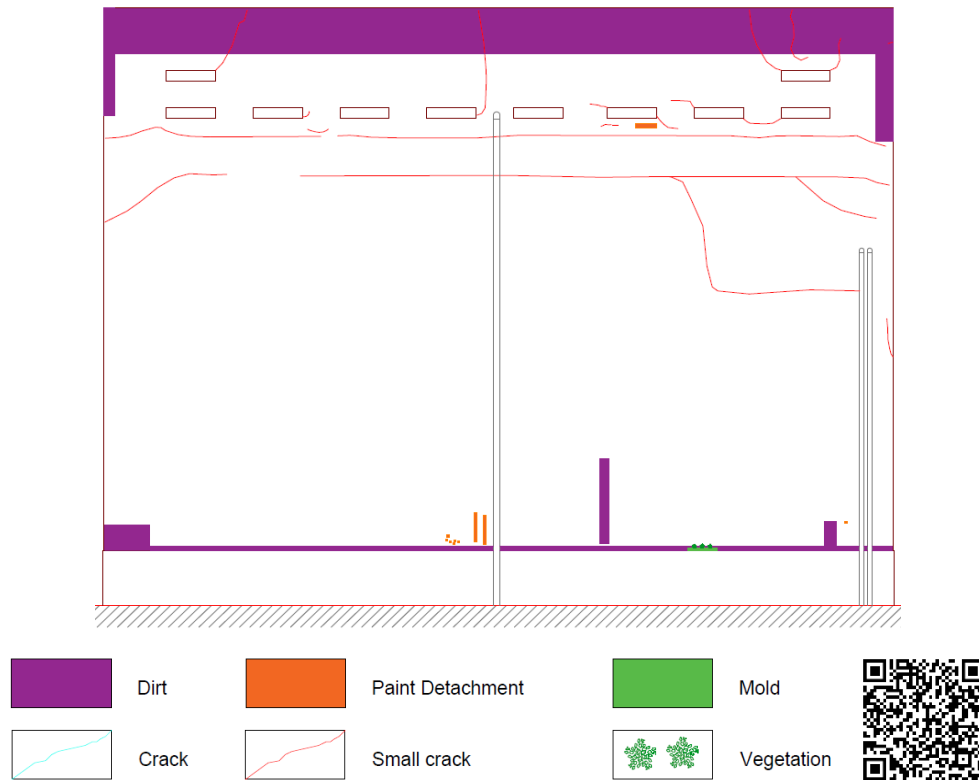
Figure 23. Damage map of the left lateral facade of block G
