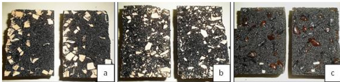
Figure 2. Specimens after failure: a) M1 mixture (SACC-D), b) M2 (SACC-S) and c) M3 (Pebble-DS).
