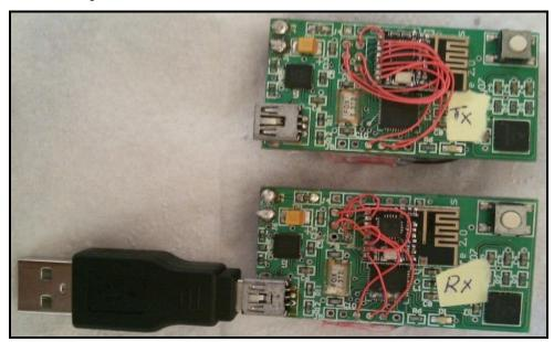
**Figure 3.** nCor 2.0 wearable wireless sensor the top one is the transmitter which is connected on the table tennis player's wrist and the bottom is the receiver going to the USB port of the coach tablet.
