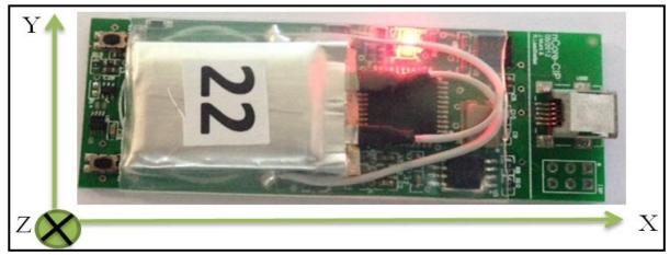
Figure 2. nCore 3.0 wearable wireless sensor.
