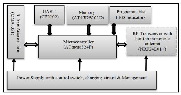
**Figure 1.** Block diagram of the nCore 2.0 & 3.0. The dotted line block represents the module that is added to the wearable wireless sensor nCore 2.0 [3-7].
