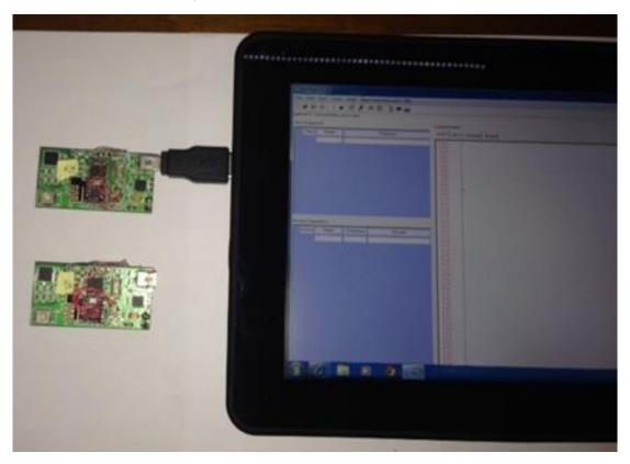
**Figure 5.** The transmitter and the receiver sensors with the coach's tablet.
