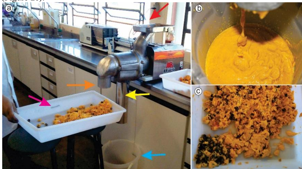
Figure 2: a) Pulp machine used in the process: place where the fruits are inserted (red arrow), place where the waste comes out (orange arrow), place where the pulp comes out (yellow arrow) and place where the pulp is being deposited (arrow blue); b) Pulp obtained in the process; c) Waste obtained in the process.
