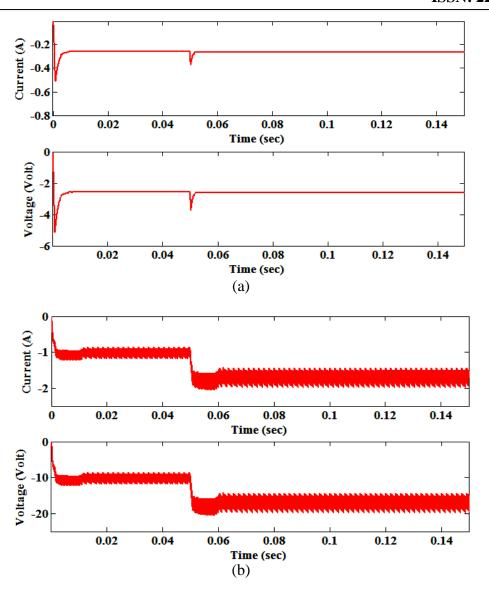
Figure 8. Dynamic response of current and voltage in Buck-Boost Converter at 30% and 70% duty cycle for  $V_g$  varies from 9V to 15V and R at  $10\Omega$ .
