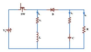
Figure 3. DC-DC buck-boost converter
