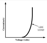
**Figure 1**. I-V characteristics of LED load.
