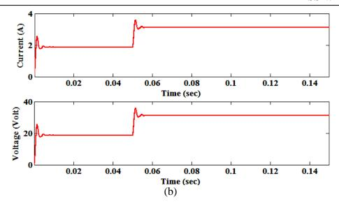
Figure 6. Dynamic response of current and voltage in SEPIC Converter at 30% and 70% duty cycle for  $V_g$  varies from 9V to 15V and Rat  $10\Omega$ .
