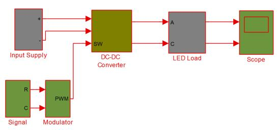
Figure 5. MATLAB-SIMULINK model of Buck-Boost/SEPIC Converter
