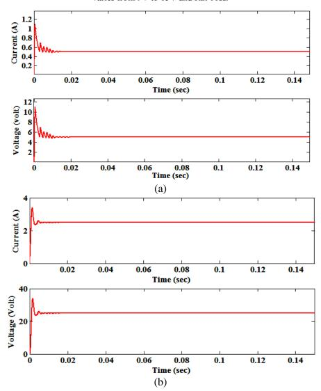
Figure 7. Dynamic response of current and voltage in SEPIC Converter at 30% and 70% duty cycle for  $V_g$  at 12V and R at  $10\Omega$ .
