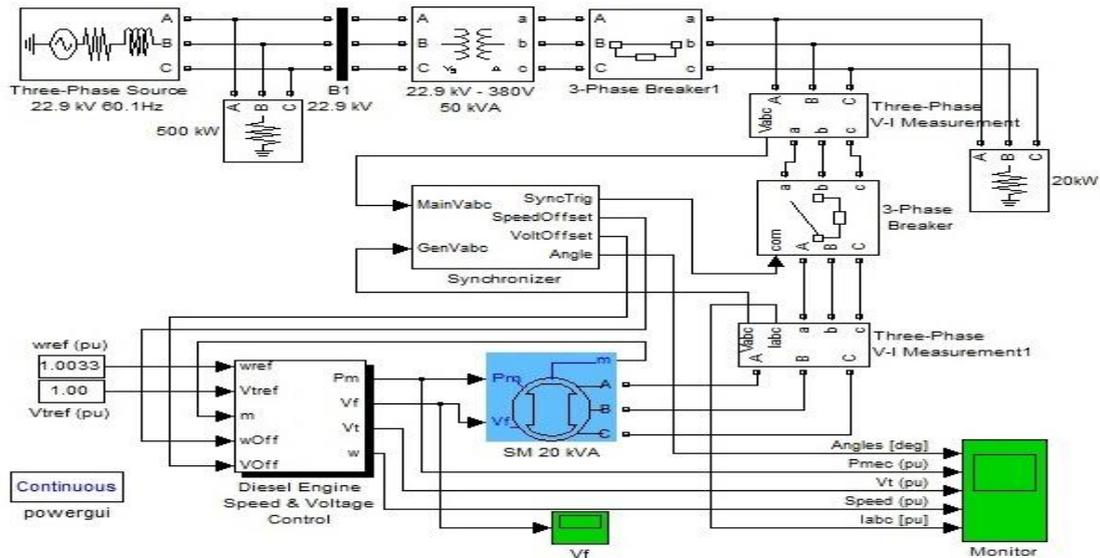
**Figure 2.** Simulation model of the diesel engine generator connected to the electric power system by the synchronizer
