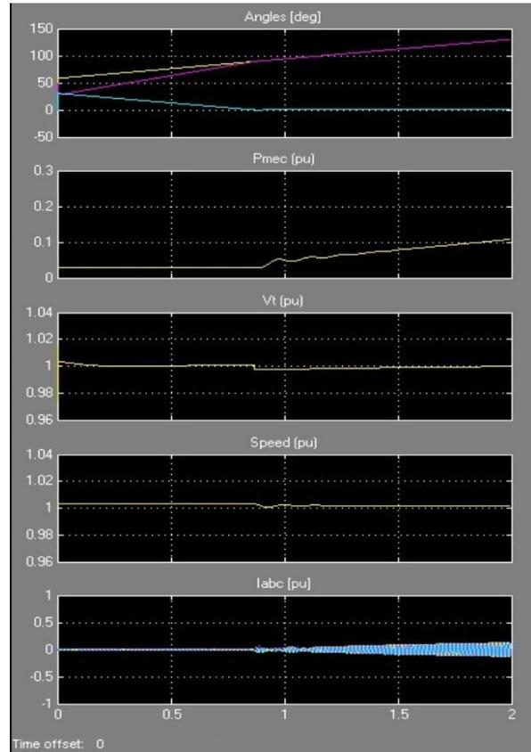
Figure 4. Case of the soft synchronizer
