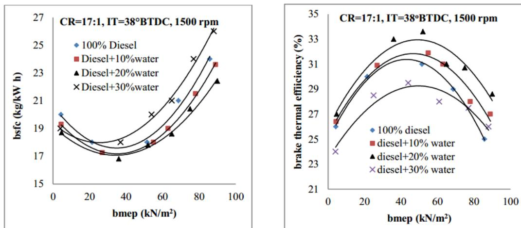
Figure 5. Effect of water-diesel emulsion in BSFC (Left) and brake thermal efficiency (Right) [4, 7]
