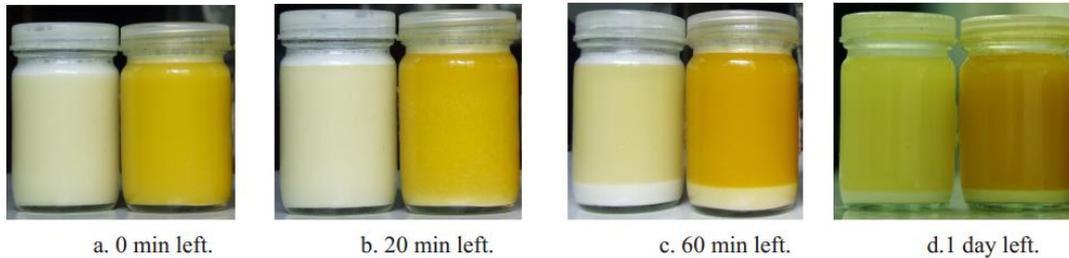
Figure 3. Water – diesel emulsion samples
