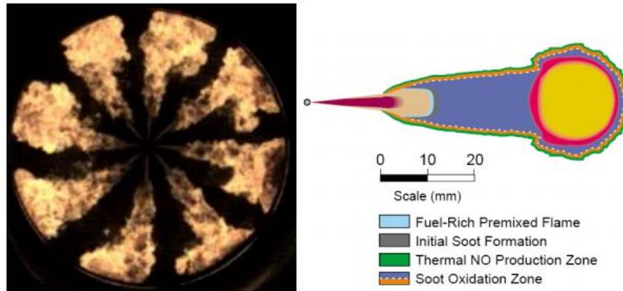
Figure 2 Diesel combustion process, [3], [4]
