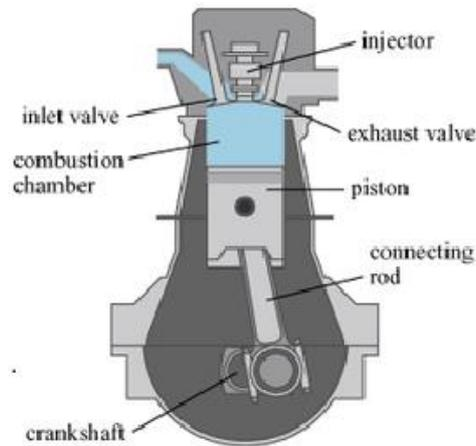
**Figure 1** shows a cross-section of a compression engine (Diesel) engine.
