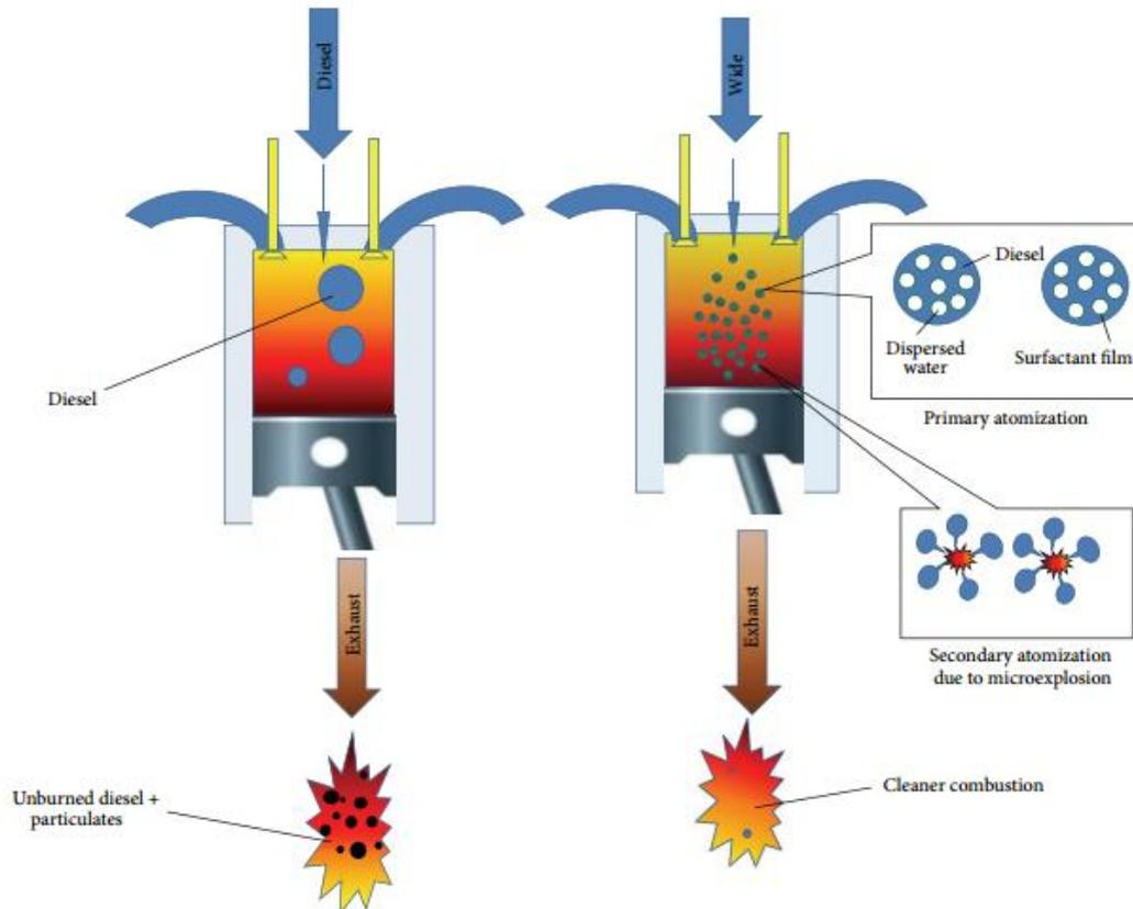
**Figure 4.** Combustion of diesel alone (Left) and the emulsion of water- diesel (right) [11]
