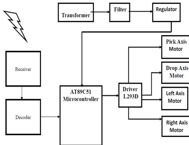
Figure2: Block Diagram of Gripper Robot
