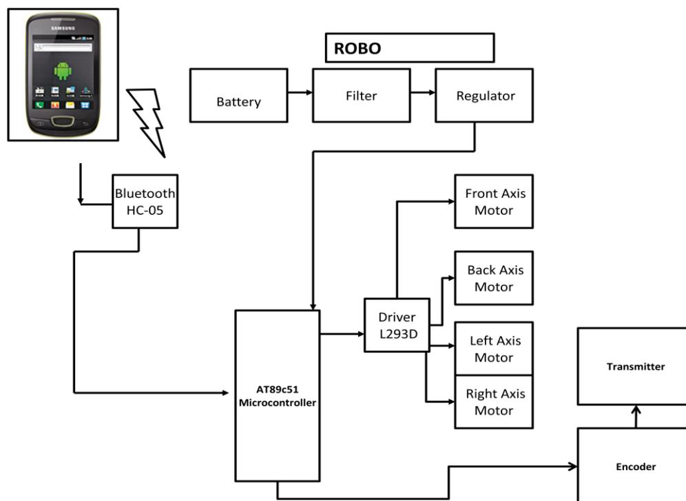
**Figure1:** Block Diagram of Moving Robot
