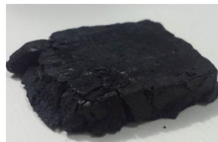
Figure 13: CBS10 after compression test
