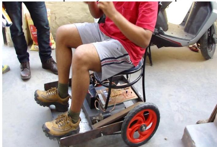
Figure 9: Head Motion controlled wheelchair
