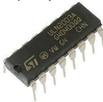
**Figure7:** ULN2003 IC used in our project
