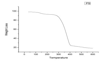
Fig. 2(a) Showing the TGA graph of FPSN film
