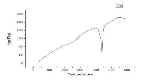
Fig 2(b) showing the DSC graph of FPSN film
